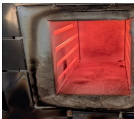
Figure 5. Furnace machine used to carbonize briquettes
