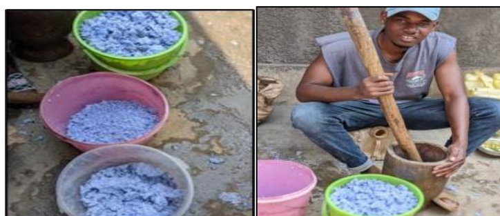
Figure 2. Grind the waste papers and reduce the amount of water
