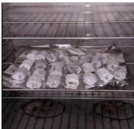
Figure 4. Allow briquettes to dry to oven
