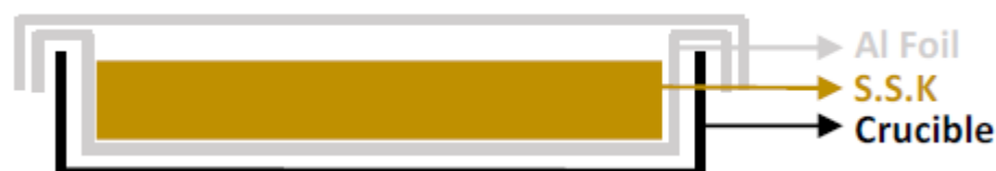
Figure 1. Foil sheet coating schematic
