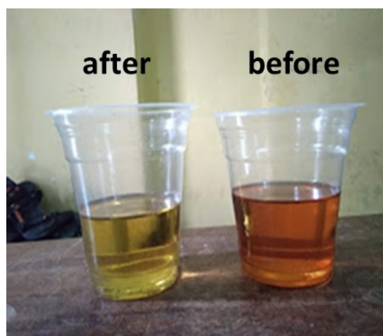
Figure 3. Changes in the color of the oil after being given a durian peel adsorbent
